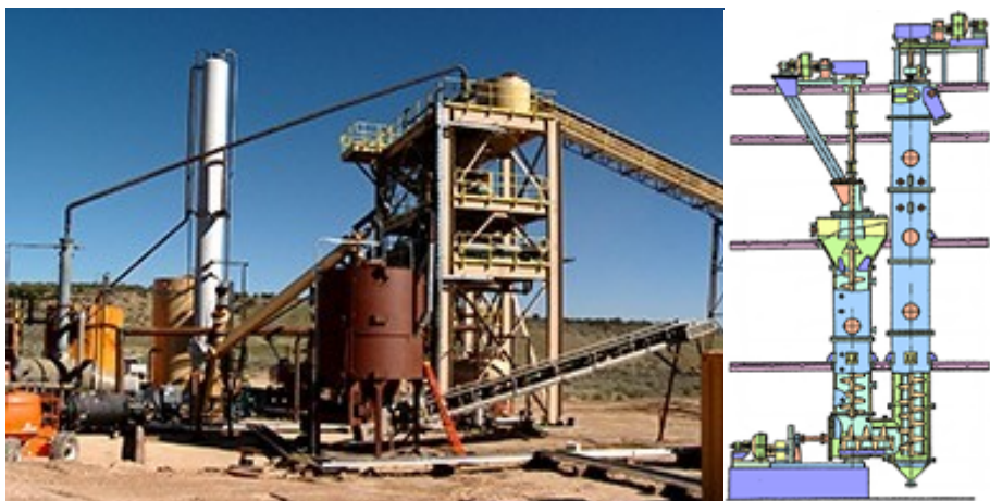
Petroteq's oil sands processing facility and schematic diagram of process. Source: Company
