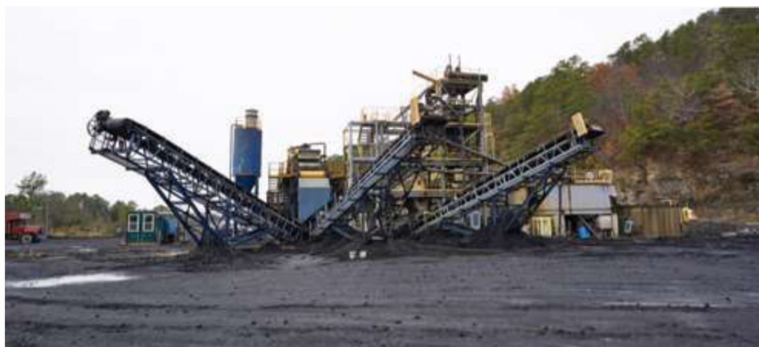
Wash plant at the Rosa Mine. Source: Company
