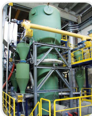
Fluidised bed gasifier using EQTEC Gasifier Technology. Source: Company
