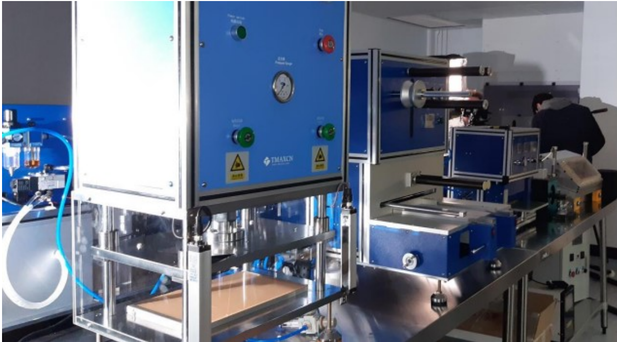
Pilot scale pouch cell production line at DGI's R&D facility in South Wales. Source: Company
