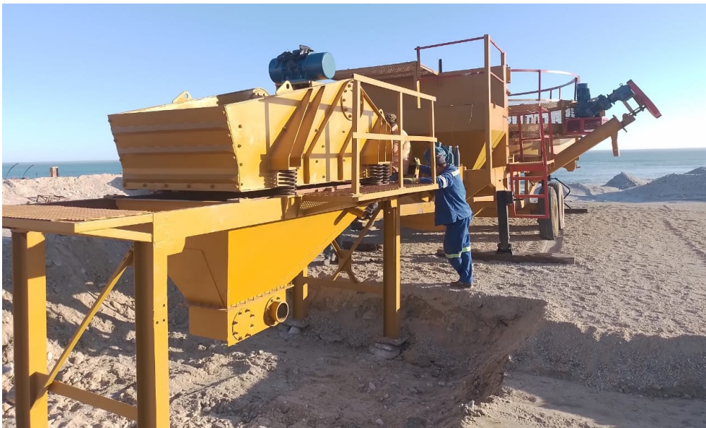
Pan Plant on site on the company's concession at Alexkor. Source: Company
